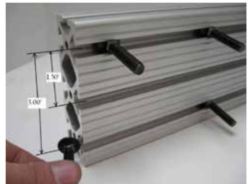
**Figure 3.1.** The heads of the included T-SLOT 5/16-18x1.5" bolts will slide into the channels found on the 80/20 aluminum base of the weld head. Use the bolts to secure the weld head to the table, with or without using the template found on page 29.
