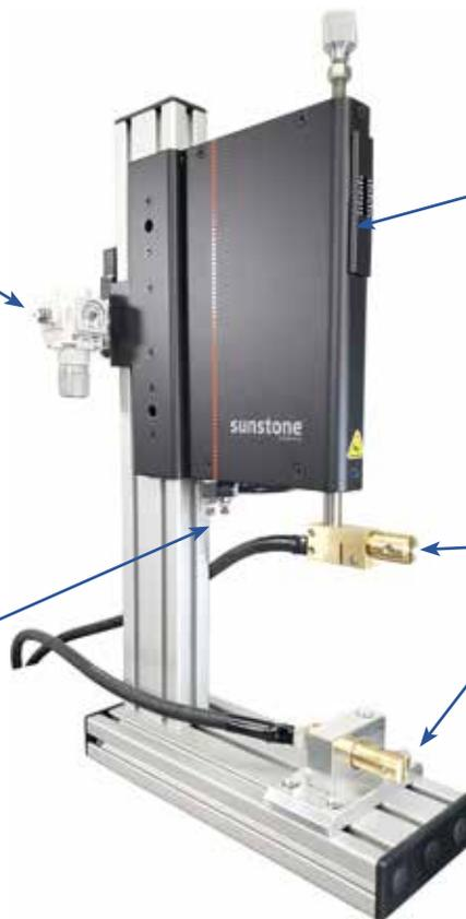
**Moveable Electrode Gap Scale.** Refer to this scale when configuring the electrode gap (the distance between the heads of the two electrodes). Follow the directions as noted in the Electrode Spring Pressure Setup section on page 17.
