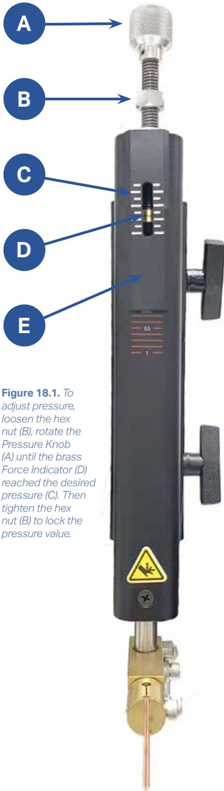
**Figure 18.1.** To adjust pressure, loosen the hex nut (B), rotate the Pressure Knob (A) until the brass Force Indicator (D) reached the desired pressure (C). Then tighten the hex nut (B) to lock the pressure value.
