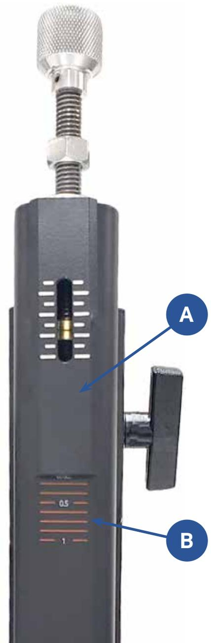
**Figure 17.1.** Set the Moveable Scale to the same height between the top electrode and the work piece.
