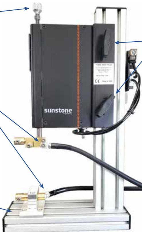
**Height Adjustment.** Loosen these knobs to move the weld head up and down when positioning the electrodes above the work piece. Sunstone suggests you start with a gap of 1/8" (0.125 inches) above the work piece.
