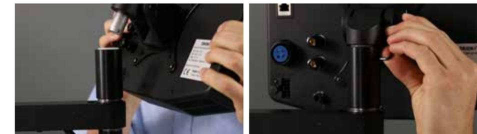
Insert the welder into the top of the arm. Then use an Allen wrench to secure the welder in place on the arm.
