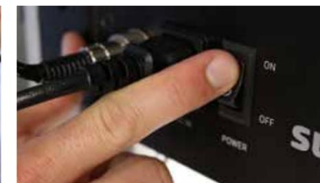
Turn on the welder with the button on the bottom of the welder, then turn on the weld head with the switch found on the side. Once both are powered the welder interface should display the EV mode tab. If you don't see this tab you may be missing a connector or may have not powered the weld head.
