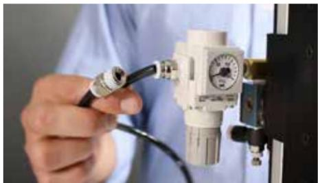
Plug the tube from the compressed air tank into the air valve system on the back of the weld head.
