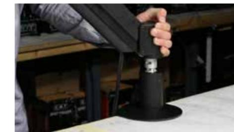
Insert the bottom end of the microscope arm into the microscope arm table mount.
