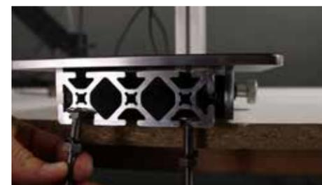
Pull the cap off the front of the weld head base. Drill four holes into your table top. Slide the screws into the base, then lower the weld head into the screw holes. This will ensure your weld head will be secured in place during welding.
