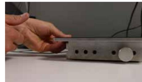
Now slide the base plate onto the base of the weld head and tighten the wheel on the side of the base plate to secure. Then replace the base plate cap.
