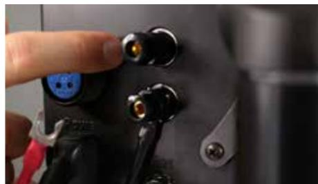
Using the wires on the weld head, connect the red wire to the positive port and the black wire to the negative port.
