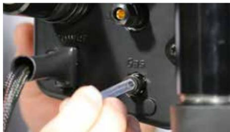
Insert shield gas hose from the argon gas regulator into the back of the welder. It will stop when it is fully connected. Tug gently on the tube to verify a tight fit.
