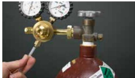
Insert the gas tube into the regulator. It will stop when it is fully connected. Tug gently on the tube to verify a tight fit.
