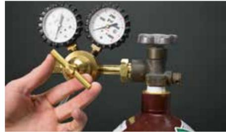
Slowly turn the regulator knob **CLOCKWISE** until the gas pressure reads between 7-10psi. The dial on the left side of the regulator should adjust.
