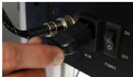
Plug the AC power cable into the side of the weld head. Then plug the other end into any standard 110-220VAC outlet.
