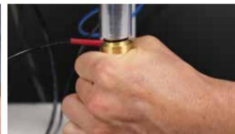
Remove the nose cap from the weld head and twist the electrode holder counter clockwise to open the collet. Insert the electrode into the collet. Tighten the electrode holder clockwise to secure the electrode in place. The electrode should protrude about a half inch out of the holder. Now replace the nose cap. \*When welding, the tip of the nose cap should be 1/8" above the work piece.
