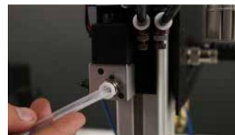
Using the provided splitter, plug the tubes into the gas port on the back of the welder and into the port on the back of the weld head at the bottom of the air valve.
