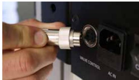
Plug the 4 DIN Connector on the back of the Weld Head into the Valve Control port on the side of the Weld Head.
