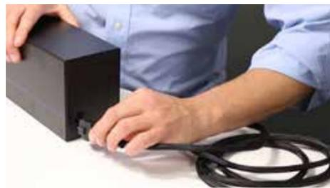
Plug the power cable into the back of the welder and to the power supply box. Now plug the AC power cord into the power supply box. Last, plug the end of the AC power cord into any standard 110-220VAC outlet.
