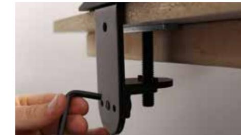
The Orion microscope arm table mount will clamp to any table top. Simply place the table mount on your tabletop in the desired location and then tighten the screw located at the bottom of the table mount with an allen wrench. Align the table mount screw with the center hole of the included steel plate and then tighten. This steel plate will help spread the weight of the system and provide more support.
