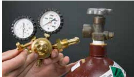
Turn regulator dial **COUNTER CLOCKWISE** until it is fully backed out to prevent over-pressurization of the line.
