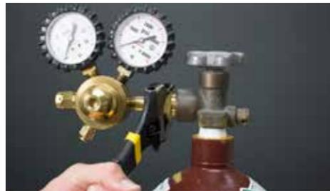
Screw the gas regulator onto the shielding gas tank.
