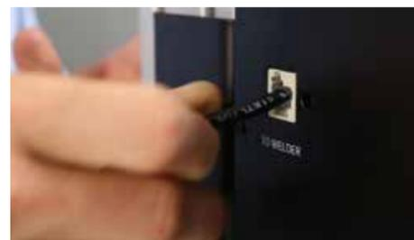
Plug the RJ-11 cable into the Acc. Port on the back of the welder then to the port on the weld head that reads "to welder".
