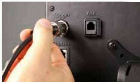
Plug the 3 DIN foot pedal connector into the port on the back of the welder marked "Trigger".
