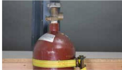
Secure gas tank to a stationary point near the welding area.
